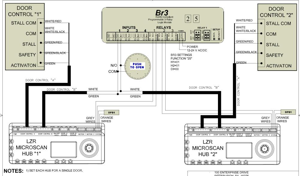
2) DOOR CONTROL "A" HARNESS FROM EACH HUB WILL GO TO IT'S RESPECTIVE CONTROL. DOOR CONTROL "B" HARNESS FROM EACH HUB WILL GO TO THE OPPOSITE CONTROL. IN THIS CONFIGURATION DOORS WILL STALL INDEPENDANTLY.
