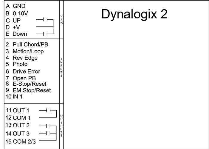
**NOTES:** 1. The activation field(s) will wire to the terminal block that is connected to the Dynalogix 2 board
