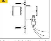
Adjust switch height on bracket until the cam triggers positively when rotated.
