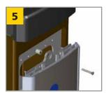
To bollard-mount (wireless versions only), attach the switch to the bollard using a 10-24 x 0.75 mounting screw and nylon spacer.
