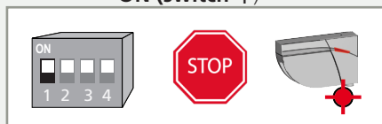
RELAY 1: STOP-impulse on swing side of door
