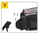
Remove Blank Endcap closest to door hinge on each sensor.
