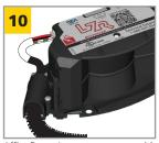
Affix Door Loop to sensor with Pass-Through Endcap and three (3)
