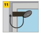
Mount the sensor to the arm. Plug the slave sensor harness into the sensor. Route Master Harness, and then install Door Loop and Cap onto the jamb
