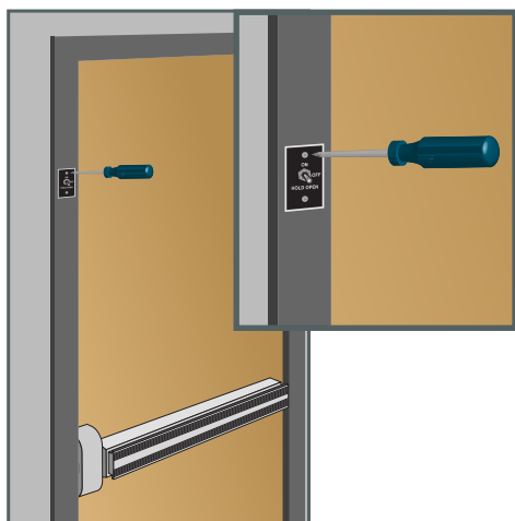
ON / OFF / HOLD OPEN Switch installed
