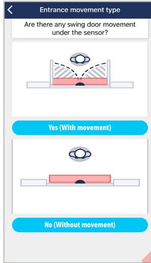
Choose if the sensor is installed above an area where there will be swing door movement.
