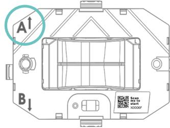
3. Remove the counting head by unclipping it.
