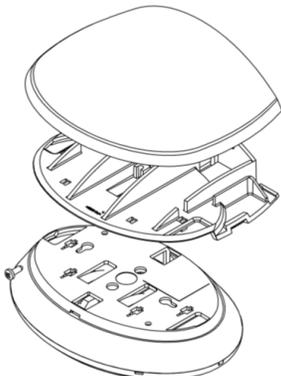
8. Connect the cable to the counting head. Clip the counting head to the base and close SIGMA.
