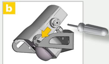
Position the sensor on the bracket and tighten the screws.
