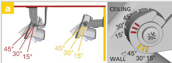
Adjust the angle of the sensor to position the detection fields.
