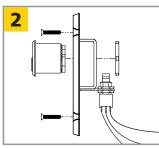
Adjust switch height on bracket until the cam triggers positively when rotated. 3 (NO) (COM) (NC)
