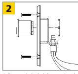
Adjust switch height on bracket until the cam triggers positively when rotated
