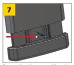
Secure the plate assembly using the bottom mounting screw. Remove the top end screw from base and slide down.
