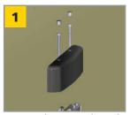
Remove the top end cap by removing its screw covers and then removing the screws.
