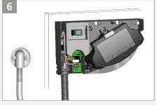
Tighten the other side of the flexible tube using the cable cap and pass through the remaining length of the power cable towards the door controller.
