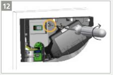
Secure the lock screw to avoid vibrations during door movement.
