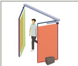
Check the correct positioning of the safety fields by walk-testing according to ANSI 156.10 standards.
