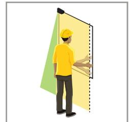
The LED will then turn green to indicate that it is time to begin the hand-gesture setup. Trace the leading edge of the door to learn the door width. The LED will blink red to indicate that the width is learned. NOTE: The sensor will automatically learn the height.
