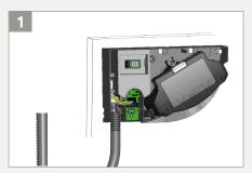
Determine the appropriate length for the door loop.
