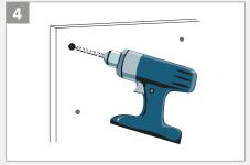
Remove the base and drill 1/8" pilot holes.
