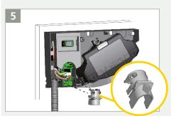
Secure the door loop to the sensor, using the clamp. Secure the 2 screws to avoid pulling out the cable.
