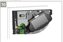
Connect the black plug to the black connector. Ensure that all wires are secured within the notch to avoid damage from the cover.
