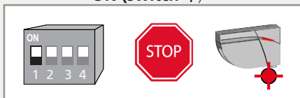
RELAY 1: STOP-impulse on swing side of door
