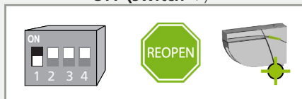
RELAY 2: REOPENING-impulse on approach side of door
