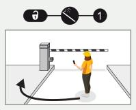
Launch a teach-in using the remote control and be sure to remove yourself and any other potential disturbances from the field within 3 seconds.
