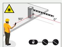
Activate the visible laser beams by remote control.
