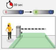
The Motion Field LED will flash red for ~30 seconds while the sensor learns the motion field environment.
