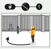
Launch a teach-in using the remote control and be sure to remove yourself and any other potential disturbances from the field within 3 seconds.
