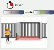
The Presence Field LED will flash red for ~30 seconds while the sensor learns the presence field environment.
