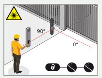
Activate the visible laser beams by remote control.
