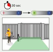
The Motion Field LED will flash red for ~30 seconds while the sensor learns the motion field environment.
