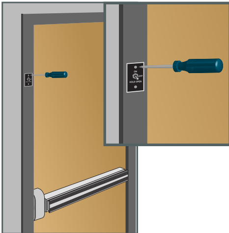
ON / OFF / HOLD OPEN Switch installed
