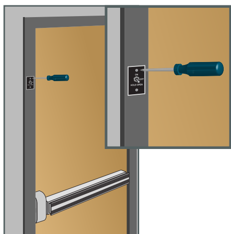
Interruptor ON / OFF / HOLD OPEN instalado
