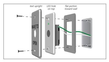
5. Secure with the provided screws (#6-32 flathead) and test functionality.
