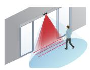
Dual Slide - Standard Door Package showing Enhanced Safety curtain position
