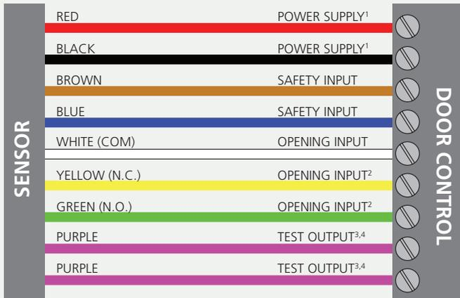
1. Voltage: 12 – 24 VAC, 50/60 Hz; 12 – 30 VDC; < 3.2 W (max)
