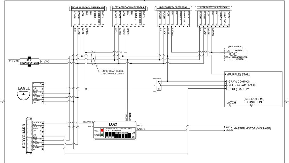
NOTES: 1 ) THE MAGNETIC REED SWITCH SHALL OPEN AT APPROX. 65-70 DEGREES TO INHIBIT THE SWING SIDE SUPERSCANS AND SHALL STAY OPEN UNTIL CLOSING CYCLE OCCURS AND THE SWITCH MAKES AT 65-70 DEGREES.
