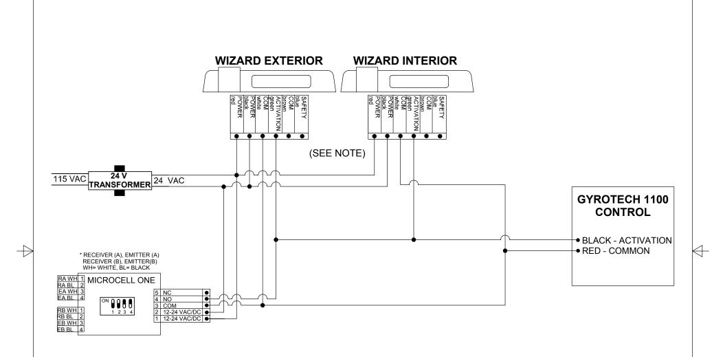
NOTE: 1) WIZARD II OUTPUT MUST BE REDIRECTED BY USING THE REMOTE. PRESS UNLOCK, F1, 1, LOCK, LOCK. THIS WILL ENSURE THRESHOLD PROTECTION IS ENABLED.
