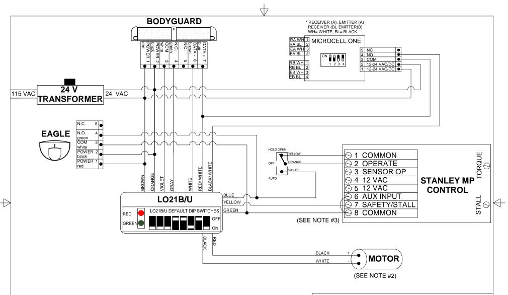
NOTES: 1) LO21U DIPSWITCH SETTINGS #1-5 (LOCK-OUT TIME), #6 (DOWN/ON), #7 (UP/ OFF), #8 (DOWN/ ON). 2) SHOWN LH,RH MAGIC SWING AND RH MAGIC FORCE FOR LH MAGIC FORCE REVERSE LO21B/U RED AND
