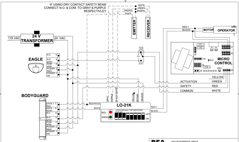
NOTES: 1) WIRE LO-21 RED / BLACK WIRES TO MICRO-SWITCH WHEN STACK OR LATCH ASSIST FUNCTIONS ARE TURNED ON. (SEE NOTE 2)
