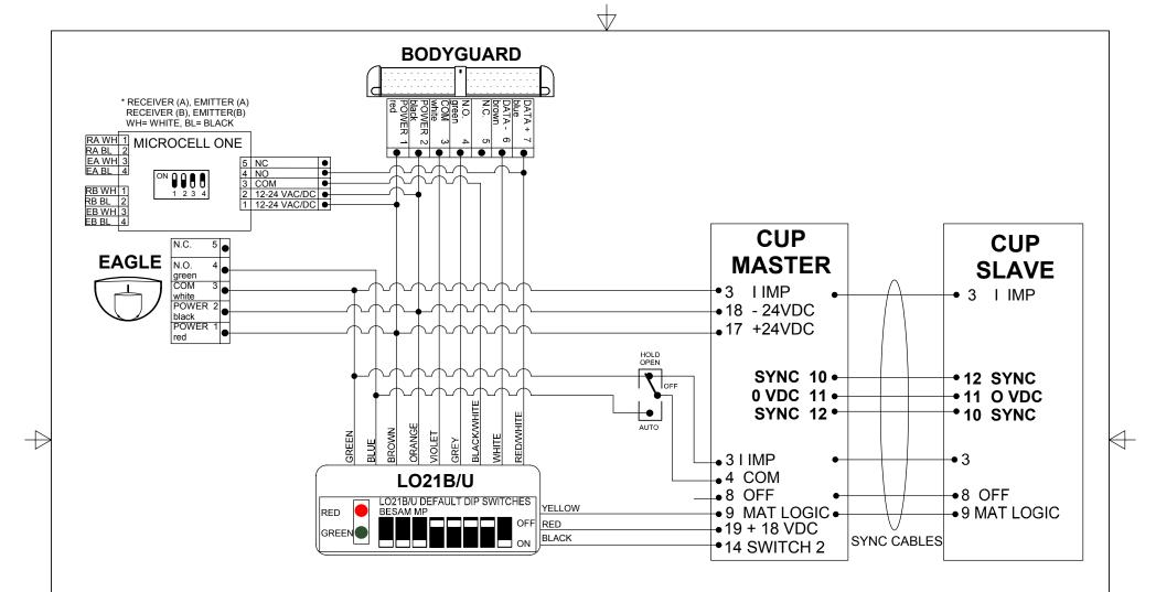
NOTES: 1) SET PMD FUNCTIONS F20 = a, F19=b, F18=00, F17=00, F16=05, F14=a, F13=a, F12 = 3 DEGREES LESS THAN F10. 2) LO21B DIPSWITCH SETTINGS #1-5 LOCKOUT TIMING, #6 UP/ OFF, #7 UP/ OFF, #8 DOWN/ ON
