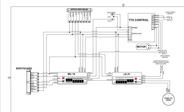
NOTE: 1) ENSURE THAT A MINIMUM OF 3 SECONDS OF HOLD OPEN TIME IS LEFT ON THE LE-21.
