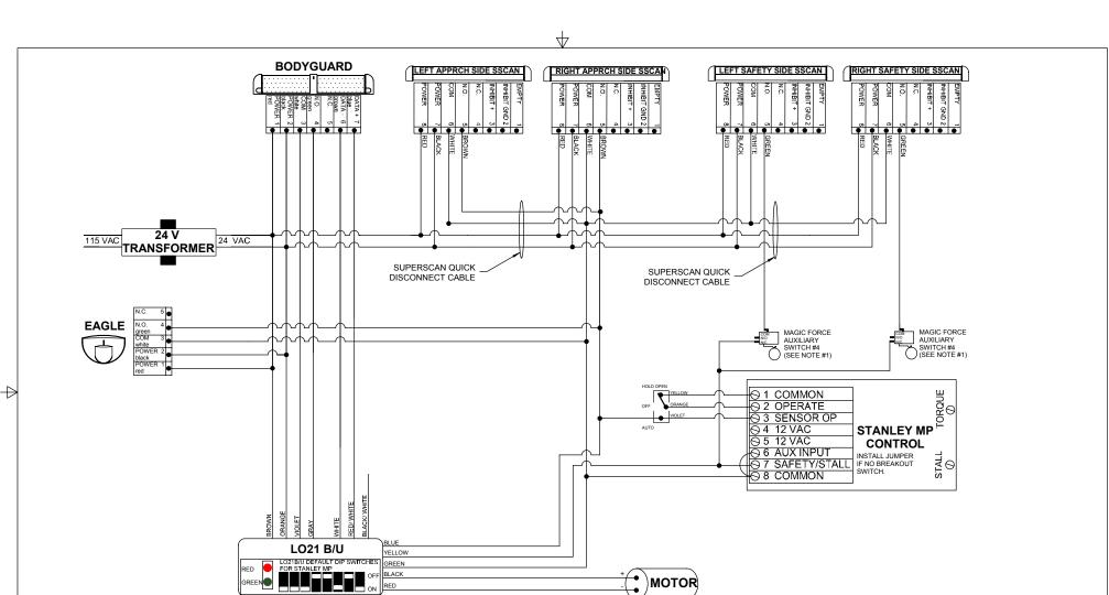
NOTES: 1 ) MAGIC FORCE AUX. SWITCH #4 SHOULD OPEN AT APPROX. 65-70 DEGREES. FOR MAGIC SWING REFER TO INHIBIT SWITCH BEA PT# 10 SSINHL OR 10SSINHR
