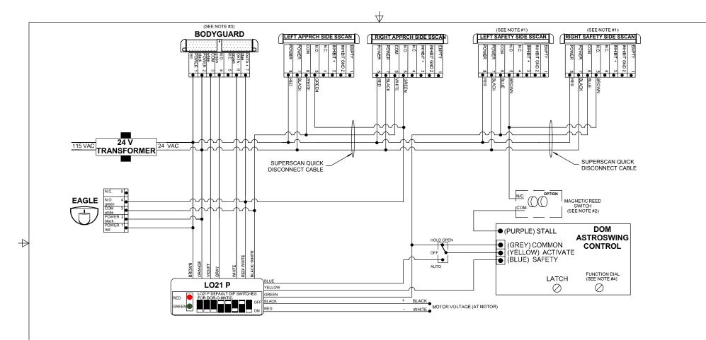
NOTES: 1 ) INSERT SAFETY SIDE SUPERSCAN BLUE WIRE INTO PIN 6, BROWN WIRE INTO PIN 5, AND WHITE WIRE INTO PIN 1.
