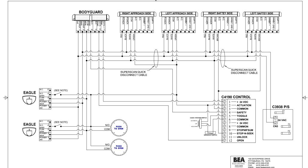
NOTE: SWITCH MUST OPEN 10 DEGREES FROM DOOR CLOSING
