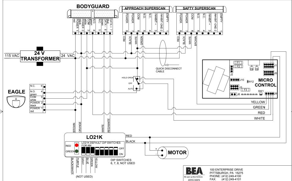
NOTES: 1) SW-1 SETTINGS (UP IS OFF) 1.PUSH-N-GO(OFF). 2. LATCH ASSIST(OFF). 3. RATCHET FUNCTION(OFF). 4. STACK PRESSURE(OFF).
