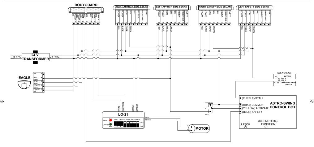
NOTES: 1) IF BODYGUARD HAS DOM INTERFACE CIRCUIT BOARD, IT MUST BE REMOVED.
