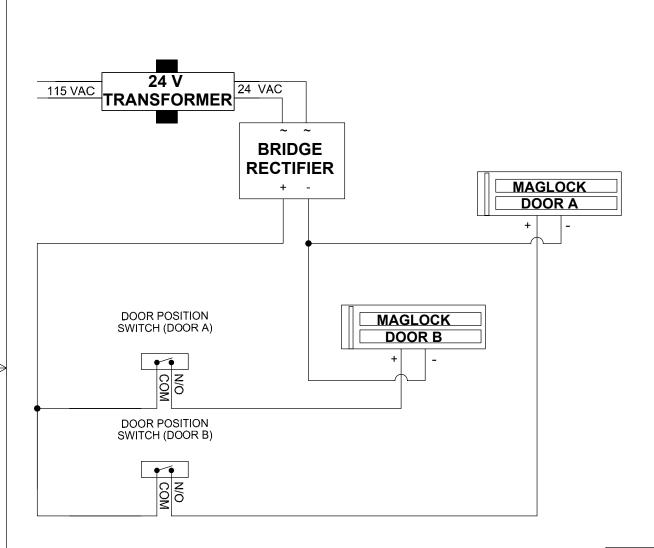
NOTES: 1) DOOR POSITION SWITCH CONTACTS MUST BE OPEN WHEN DOOR IS CLOSED. DOOR POSITION SWITCH CONTACTS MUST BE CLOSED WHEN DOOR IS OPEN.
