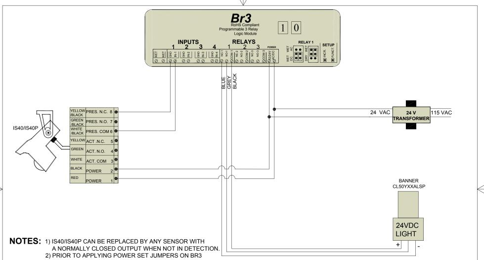
PRIOR TO APPLYING POWER SET JUMPERS ON BR3 FOR A "WET / D.C." OUTPUT.
