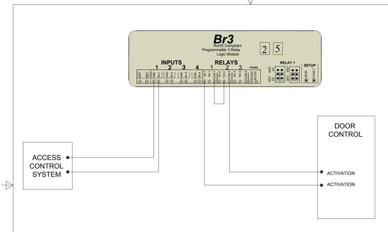
SCENARIO: ACCESS CONTROL SYSTEM HAS A RELAY OUTPUT THAT HOLDS FOR 2 MINUTES. YOU DON'T WANT ACTIVATION TO OCCUR UNTIL AFTER RELAY RELEASES.
