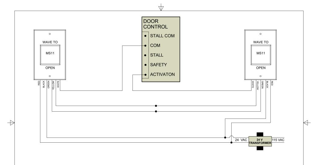
NOTES: 1) SET MS11 TO TOGGLE MODE. 2) EITHER SWITCH CAN OPEN AND/OR CLOSE THE DOOR.
