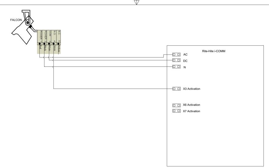
NOTES: 1. X3, X6, and X7 are programmable inputs that can usually be used for activation or "reversing edge" type action 2. For activation, set input function to 02: Activation In
