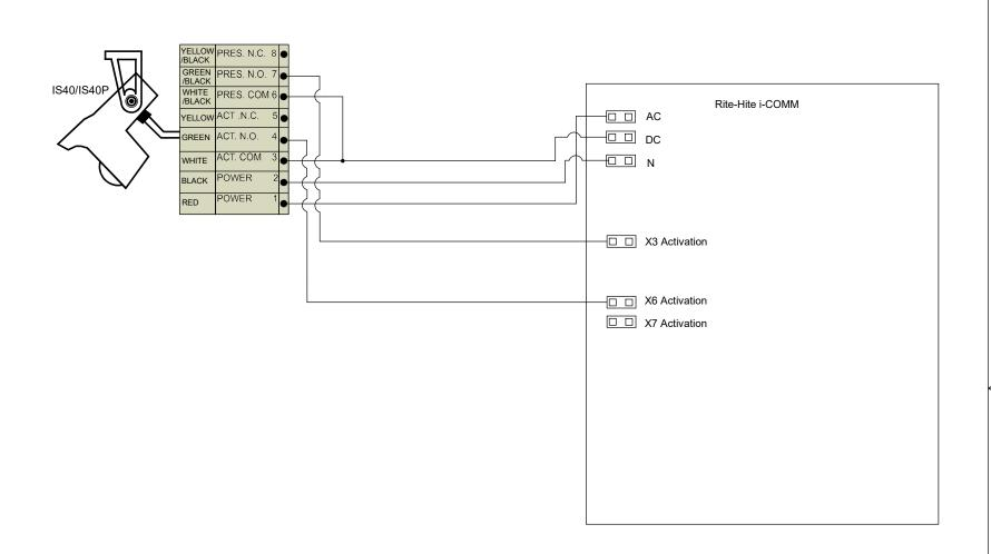
NOTES: 1. X3, X6, and X7 are programmable inputs that can usually be used for activation or "reversing edge" type action 2. For activation, set input function to 02: Activation In
