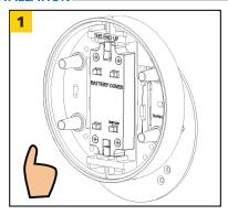
Remove Housing Assembly from Mounting Bracket by pressing in on locking tab and sliding up.
