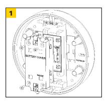
Remove four (4) screws on Battery Enclosure.
