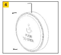
Insert Faceplate into Housing Assembly and use Hex Key to engage spring clips on the top and bottom of Housing Assembly. To remove, use Hex Key to disengage spring clips.
