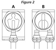
Adjust height of switch on bracket until cam triggers positively when rotated.
