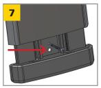
Secure the plate assembly using the bottom mounting screw. Remove the top end screw from base and slide down.
