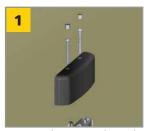
Remove the top end cap by removing its screw covers and then removing the screws.
