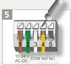
Connect the wires accordingly. 12-24 AC/DC – Brown, Green COM – White NO/NC – Yellow
