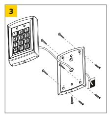
Mount backcase on the wall with provided screws. Make sure to pull keypad cable through the center hole.
