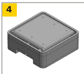
Install push plate to box.
