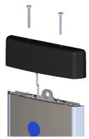
8. Fasten new top end cap and replace top end cap screw covers (from step 1)
