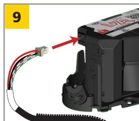
9 Route "Y" Harness through Door Loop and plug into sensor at closest port.
