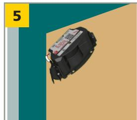
5 Using instructions on Mounting Template, mount sensors with appropriate screws. **DO NOT APPLY COVERS UNTIL SYSTEM IS FULLY OPERATIONAL.**
