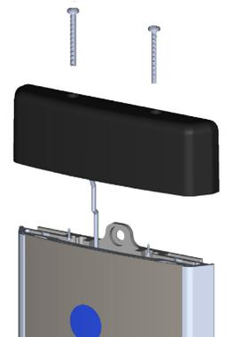
8. Fasten new top end cap and replace top end cap screw covers (from step 1)
