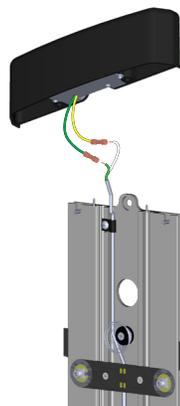
6. Insert wires into butt connectors leading from new top end cap (included) and crimp
