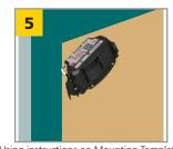
Using instructions on Mounting Template, mount sensors with appropriate screws. DO NOT APPLY COVERS UNTIL SYSTEM IS FULLY OPERATIONAL.
