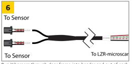
Run Y-harness through door frame into header and out of each wire passage hole in jamb. Y-harness must be run through door frame prior to inserting it through door loops and plugging into sensors.
