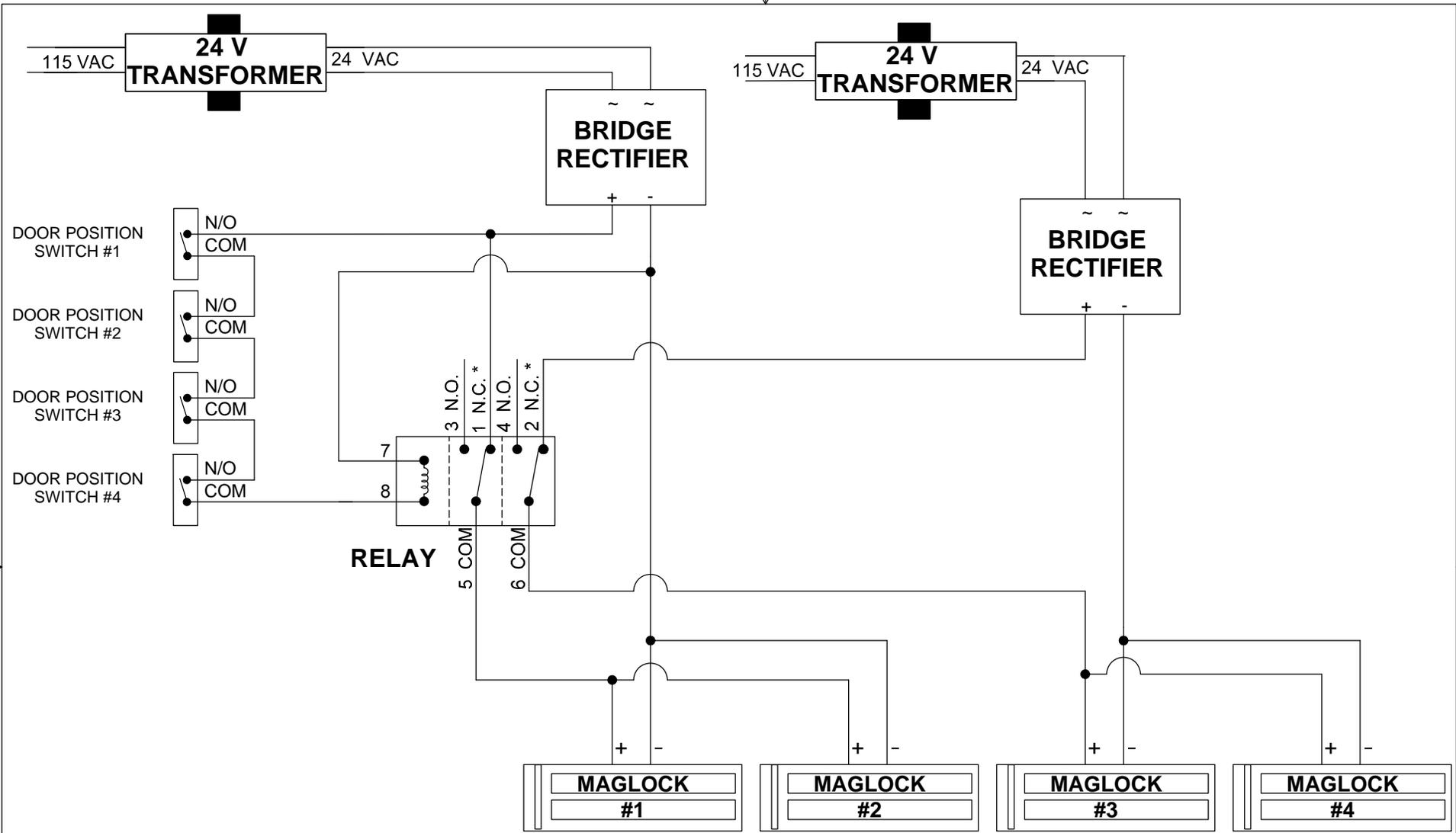
NOTES 1) DOOR POSITION SWITCH CONTACTS MUST BE CLOSED WHEN DOOR IS CLOSED. DOOR POSITION SWITCH CONTACTS MUST BE OPEN WHEN DOOR IS OPEN.
