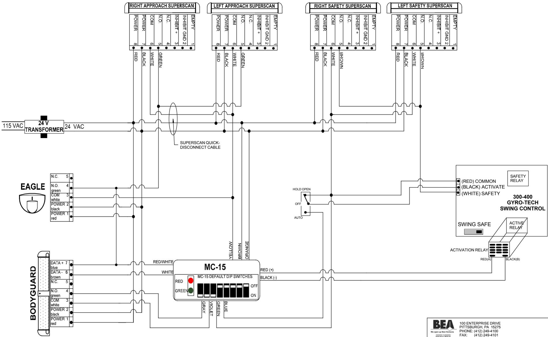
NOTES: 1) MUST SLIDE SWITCH ON CONTROL TO "SWING SAFE" POSITION.
