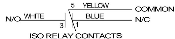
**FIGURE 1: WIRING FROM CONTROL BOX FOR BACK CHECK**
